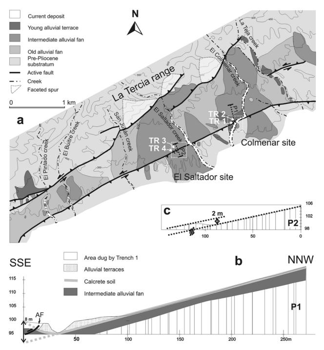
**Figure 3.** (a) Geomorphological sketch of the studied area between Lorca and Totana. Microtopographic profiles and trenches 1 to 4 are located on the map. (b) Microtopographic profile along the El Saltador fan and across the fault. (c) Geological cross section of the Colmenar site based on a microtopographical profile. Note that the offset of the calcrete soil on top of the intermediate alluvial fan is 8 m.
