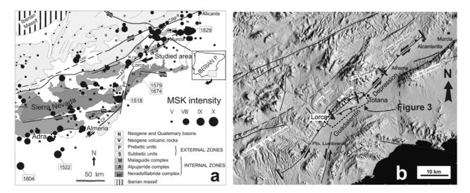
**Figure 2.** (a) Macroseismicity map of eastern Betics with the main Neogene faults. Indicated fault movements correspond to late Neogene. CRF, Crevillente fault; AF, Alhama de Murcia fault; CF, Carrascoy fault; PF, Palomares fault; CF, Carboneras fault. (b) Topographical model of the surroundings of the Alhama de Murcia fault, next to the Neogene Guadalentin depression. The segment boundaries along the Alhama de Murcia fault are indicated by black bars.
